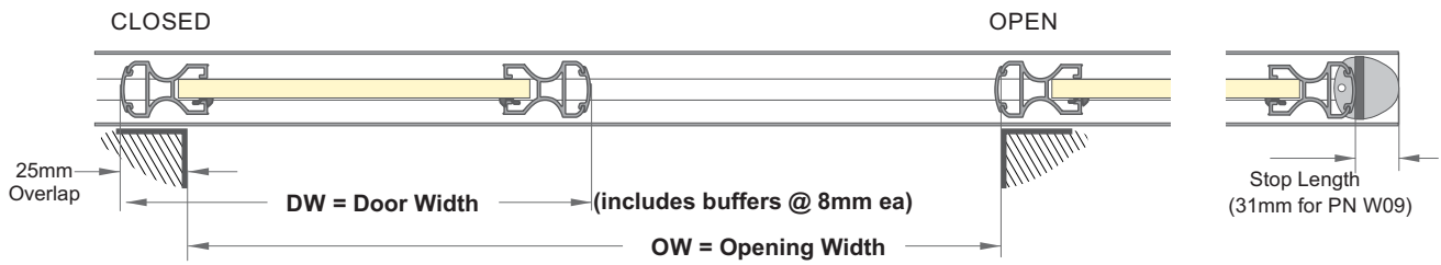
Typical Horizontal Cross Section Single Track - Face Mount
