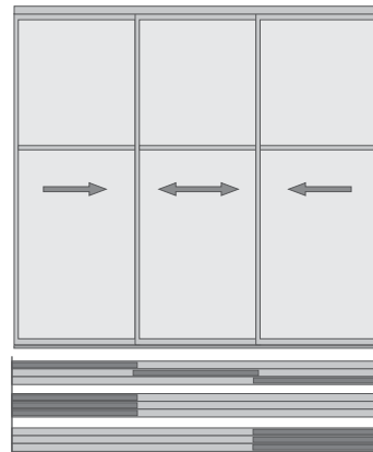
Three Panels on Triple Track (between Jamb mount)
