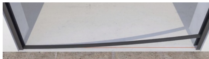
6 - After cleaning the floor area, attach Bottom Rail to the Floor with attached DS tape
