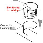
Push Fit Connector Housing can be used in non critical areas, such as middle shelves
