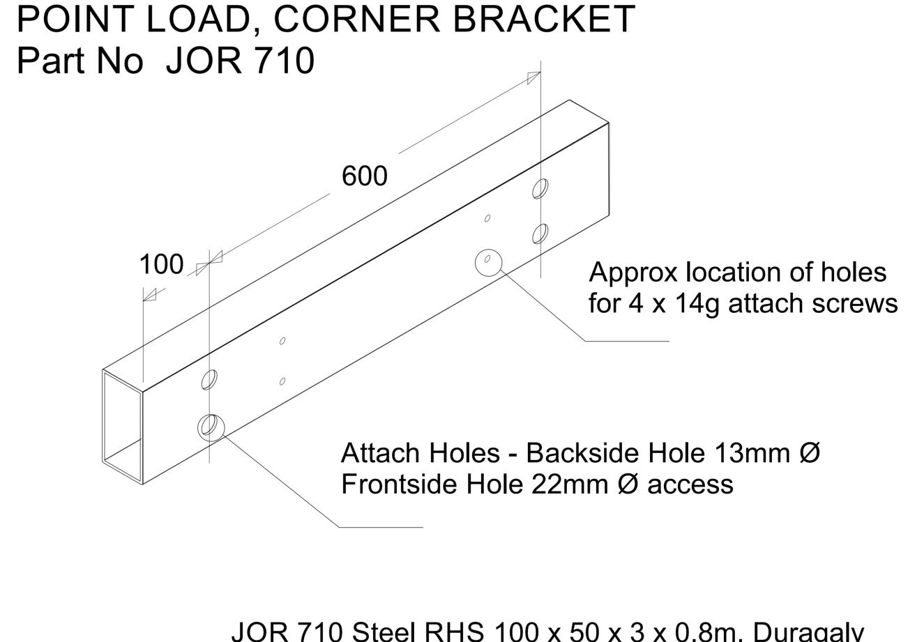
JOR 710 Steel RHS 100 x 50 x 3 x 0.8m. Duragalv securely screwed to studs or lintel with 4 x M12 SS Coachscrews. Drill attach holes to line up with studs (if needed) or use existing holes into lintel Mount hard into 507 beam corners
