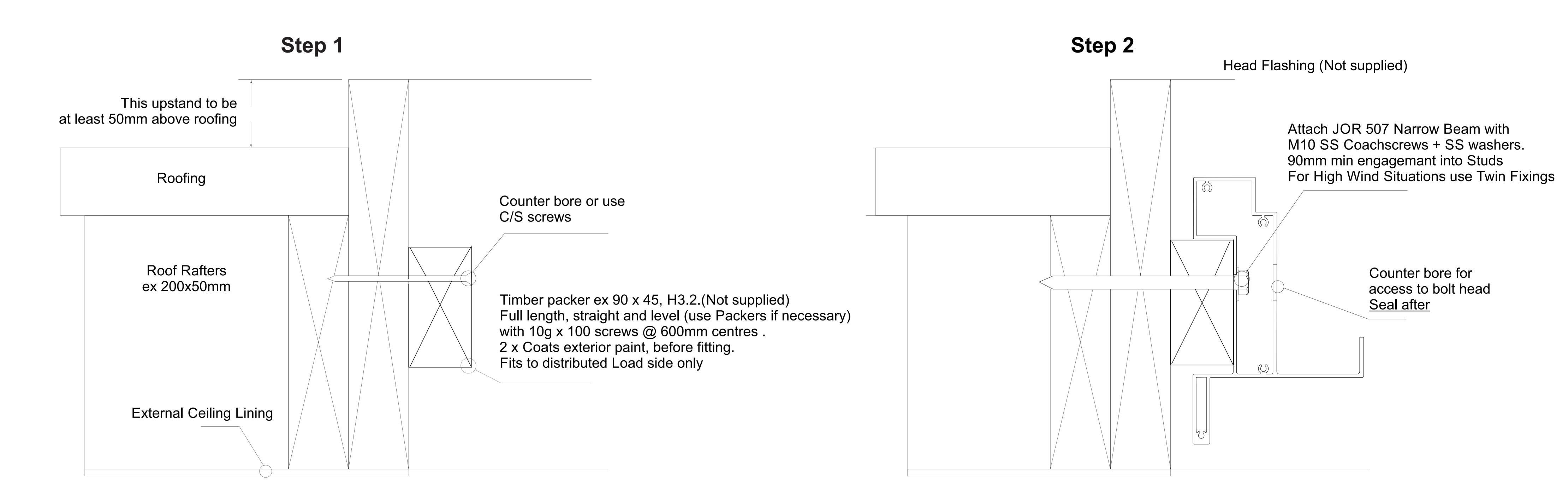
Typical Integrated Roof Construction. Boundary joists all very firmly attached to Roof rafters. Engineer to check structure
