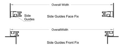
All these Horizontal Measurements, NOT using Side Wall Channel.
