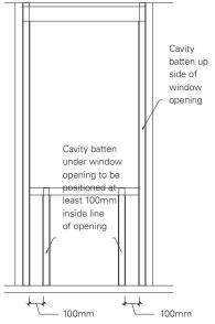
for air flow between adjacent cavities by leaving a minimum 10mm gap between the bottom of the vertical cavity batten and the flashing to the opening.
