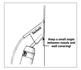
Remember to maintain a constant angle between the welding nozzle and the wall to preheat the joint properly.
