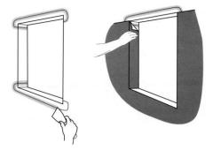
Alternative 2: At window-recesses the wall covering is rolled out over the window area and is then folded into the reveals. Loose pieces are inserted at the bottom recess, and at the top recess where necessary. The loose pieces are joined to the wall covering with welded seams.
