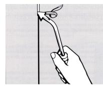
All seams are grooved using Tarkett Seam grooving Tool. Groove to about 3/4 of the thickness.
