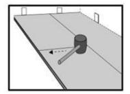
7. Start the second row by cutting the flooring to the desired length. Keep in mind that piece must not be shorter than 6" (15cm) to achieve the best appearance.
