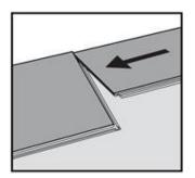
6. If needed use a rubber mallet to fully engage the short side of the flooring by lightly tapping on the top of the flooring to engage and sit flush with the adjacent piece. Maintain an expansion gap of approximately 1/4" from the wall. Repeat this process to complete the first row. If the end is raised use a non-marking rubber mallet to lightly tap the end (tongue side) about 1" from the seam. Do NOT tap directly on the seam.
