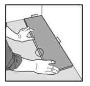
5. Install the second row by aligning and dropping the end tongue over the end groove of the first piece. Apply light pressure to join the two pieces together.
