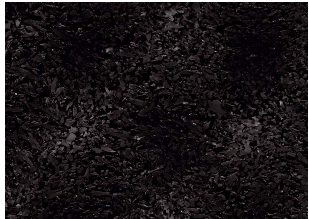
Regupol® 6010 is manufactured using recycled SBR rubber
