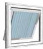
top hung window outwards opening
