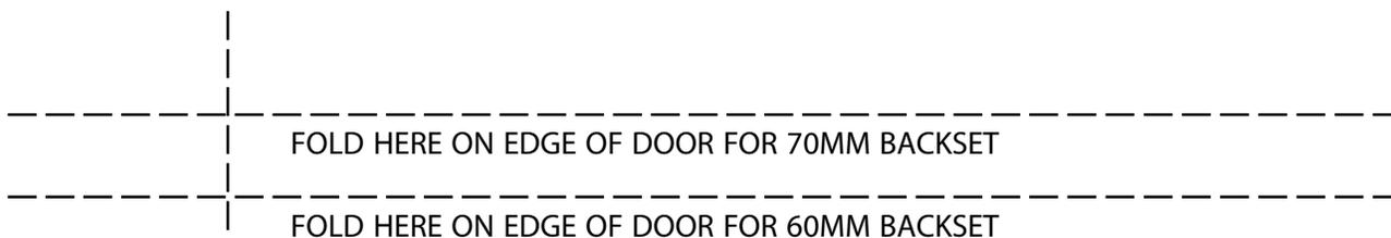
THIS WAY UP FOR RH EXTERNAL & LH INTERNAL PLATES
