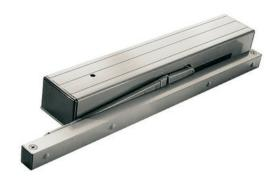
The LCN 4314ME Sentronic is a heavy duty fixed strength, electronic closer designed to provide infinitely adjustable hold open points for fire and smoke barrier doors. The door is held open until current interruption releases the holding mechanism and the door closes. Automatic detection and containment of fire and smoke are the best methods for minimising danger to life and property.
