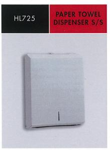
0.8mm type 304 stainless steel with a #4 Cold rolled steel with white powder satin finish. Unit fitted with tumbler lock. Dispenses 450 C-fold or 600 Multi-fold paper towels.
