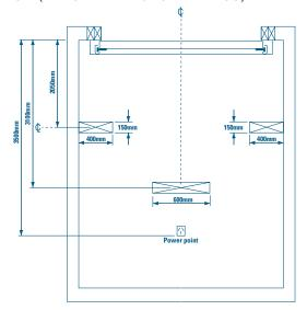
The details shown are for 2.28m Maximum height Sectional Door with Standard 330mm Headroom. Also for Intermediate Headroom of 220mm with springing to front.
