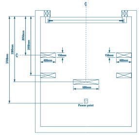
The details shown are for 2.75m Maximum height Sectional Door with Standard 330mm Headroom. Also for Intermediate Headroom of 220mm with springing to front. Measurements for motor with 2.5m C-Rail, add 1m when using a 1m extension.
