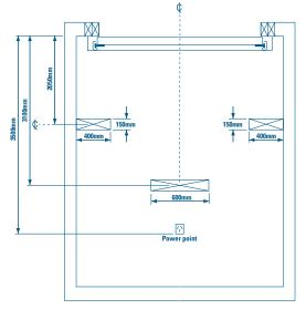
Note: The details shown are for 2.28m Maximum height Sectional Door with Standard 330mm Headroom. Also for Intermediate Headroom of 220mm with springing to front.
