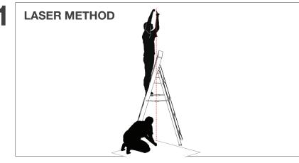
Lay supplied stencil on ground directly below ceiling surface you would like to install your Vista panel. Point laser vertically on each marked spot on the stencil while the second person marks the laser spots on the ceiling using a ladder. Apply this method to each attachment spot.
