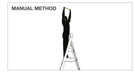
Hold stencil to ceiling, marking all fitment locations on ceiling. If unable to use stencil, use measurements marked on stencil and manually measure and transfer markings.
