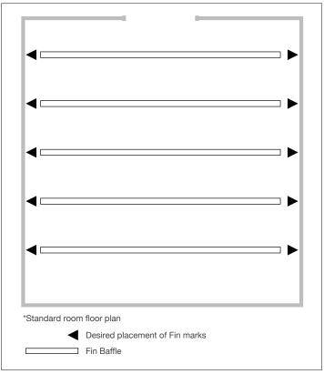
Measuring centre to centre, mark the desired placement of Fin baffles on floor.
