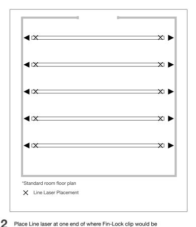
Place Line laser at one end of where Fin-Lock clip would be (See Page 2 for dimensions), projecting laser onto ceiling.
