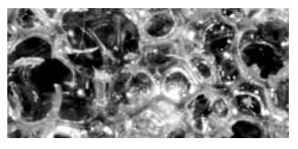
As viewed through a microscope. Polyether foams are naturally hydrolysis resistant and display excellent acoustic characteristics.
