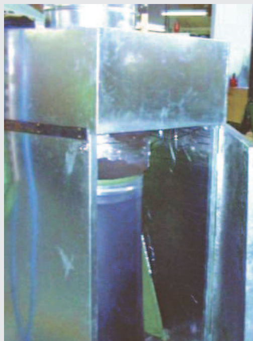
The first step in noise reduction is to consider treating the noise problem at source. This has the advantage of reducing costs and being more practical where process considerations prevent full enclosures. Acoustop MultiGrade lining allows for effective small localised enclosures
