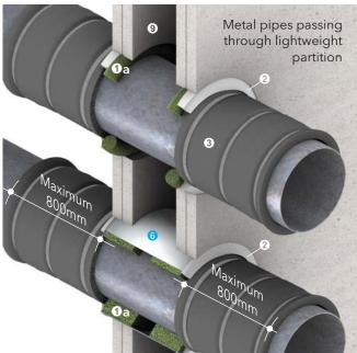
Up to -/240/240 fire resistance in accordance with the requirements of BS 476: Part 20: 1987 and/or AS 1530: Part 4: 2005, depending on applications and types of penetrating elements
