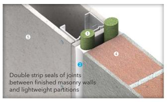
Up to -/240/240 fire resistance in accordance with the requirements of BS 476: Part 20: 1987 and/or AS 1530: Part 4: 2005, depending on applications and types of penetrating elements
