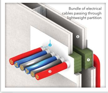
Up to -/240/240 fire resistance in accordance with the requirements of BS 476: Part 20: 1987 and/or AS 1530: Part 4: 2005, depending on applications and types of penetrating elements
