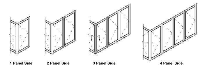
Panel numbers either side of the 90° corner can be arranged to suit most configurations, with the exception being Lay-Back Panels which can only be on a two panel side. Internal corner units are not possible.
