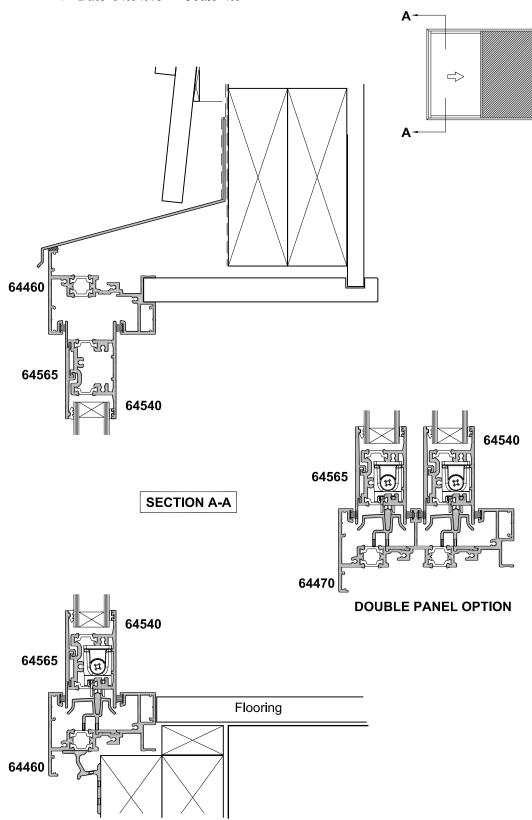
NOTE: This detail is typical only and may differ for various claddings and building in situations.
