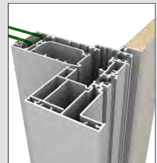
The sliding door jamb detail.
