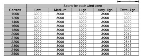
Spans are the maximum calculated allowable, based on NZS4211:2008, which requires that the member deflection at serviceability wind pressure (SWP) shall not exceed 1/200 of the span. Hardware and componentry may further restrict the spans. Spans with asterix will meet code requirements but will have max deflection greater than 18mm. For advice we recommend you contact APL Technical Advisory Service
