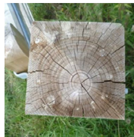
Example of solid timber checking (Softwood)
