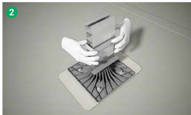
Putting in place the blocker to keep the raisers from being dislodged from the top of the pedestal.
