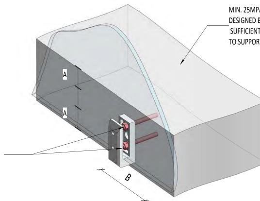
MIN. 25MPA CONCRETE MIN. 190mm THICK
