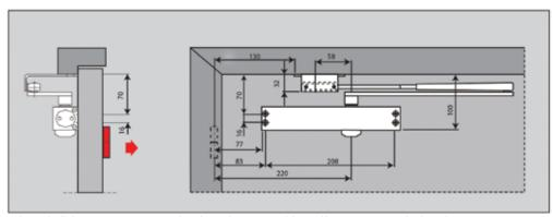
With this fixing method, the closing force is approx. 20NM (for doors up to 950mm)
