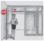
The **mechanical hold-open device** enables doors to be held without fallback at an opening angle up to approx. 120°.
