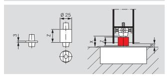
Calculating the necessary length of spindle extension: Extension =  $\mathbf{X}$  – Floor clearance (normally 8 mm) Collar height  $\mathbf{Z}$  of the extended spindle inserts = Spindle extension length + 3 mm (collar height of the standard spindle insert)
