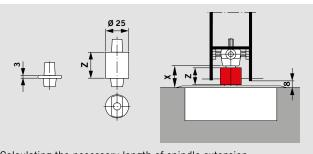
Calculating the necessary length of spindle extension:
