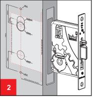
2. Important Do not attempt to drill holes whilst lock is in mortice. Drill the 4.5mm fixing holes half way through the door and repeat on the other side, with the holes meeting in the middle of the door. Drill other holes as per template that are required to match function of plates.
