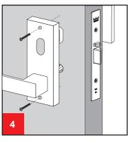
4. Insert spindle and spring supplied into lever to both sides of the door (spring locates fully into lever). Determine the correct screw length to suit the door thickness then cut screws
