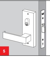
Install furniture to the door. Do not over tighten screws with excessive tension on power driver as this may damage screws and void warranty.
