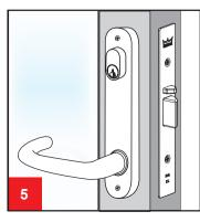
5. Install furniture to the door. Do not over tighten screws with excessive tension on power driver as this may damage screws and void warranty.
