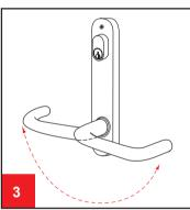
3. Non handed levers To change handing rotate lever 180°.
