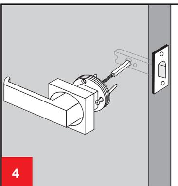
4. Insert spindle and spring supplied with levers to both sides of the door, as shown. Determine the correct screw length to suit the door thickness then cut screws.
