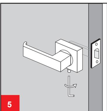
5. Install furniture to the door do not tighten screws with excessive tension on power driver as this may damage screws and void warranty. Fit and align square outer rose. Secure with grub screw from underside of rose to complete installation.
