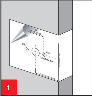
1. Position template and mark out drilling centres. **Important** also refer to lock/latch manufacturer's template prior to drilling. This template applies to bolt through fix lock/latch with a 60mm backset.
