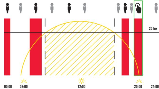
A 200° motion detector is installed on the front of a detached house. In fully automatic mode, it uses motion- and daylight-dependent light control. The user can also switch on the lighting manually from inside using a button.
