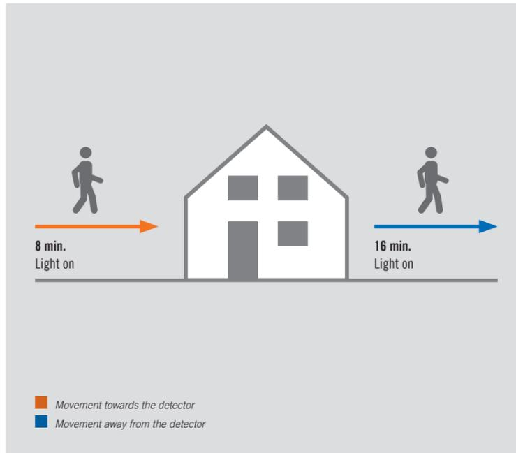
A 230° motion detector is mounted above a door area. If someone enters the house and walks towards the detector, the overrun time ends after an energy-saving 8 minutes. When walking in the opposite direction, the overrun time allows the light to shine for another 16 minutes, thus creating security through an illuminated outdoor area.
