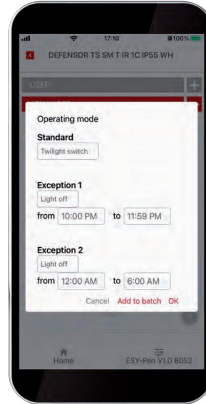
As their name suggests, the DEFENSOR twilight switches switch on the lighting when dusk begins to fall and only switch it off again the next morning once there is sufficient daylight. However, there are various scenarios in which it may be necessary to deviate from this operating mode.
