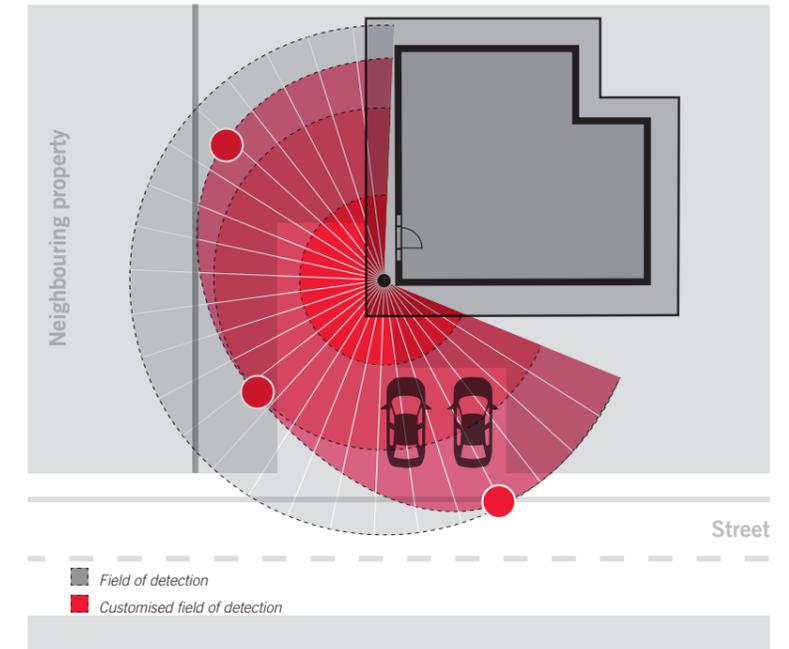
In the example, the maximum field of detection would extend to the street and to the neighbouring property, and as such would result in the lighting frequently being switched on unnecessarily. The range in these zones has therefore been reduced accordingly.
