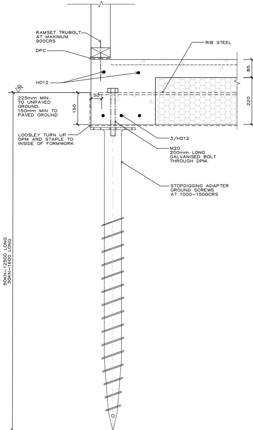
Stopdigging Groundscrews are used as an alternative to a deepened perimeter footing or cantilevered slab design in either expansive ground or ground with low bearing capacity. The ground screws extend beyond the influence of the shrink-swell zone, or low bearing capacity and support the slab edge and any point loads.
