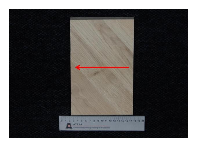
Figure 1: Finfloor Supreme - Chevron Arrow indicates direction of testing
