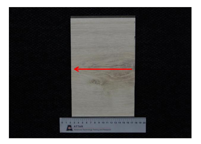
Figure 1:Finfloor XL - Wood Impression finish<br/>Arrow indicates direction of testing
