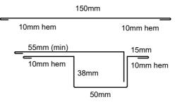
FLASHING DIMENSIONS ARE INDICATIVE ONLY AND ARE TO BE MEASURED AND DETERMINED ONSITE
