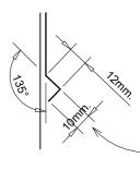
BIRD'S BEAK at bottom edge of vertical flashing Bird's beak dimension may vary between manufacturing locations.
