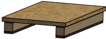
Cut & glue strips of isolation rubber and fix to hatch edges.
