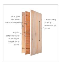
The CLT paling, manufactured by a respectable brand in New Zealand, is a cross-laminated timber plank developed using high-performance European glue lamination technology.
