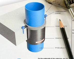
On the underside of the substrate, the TD Collar may be exposed no more than 80mm, or be recessed no more than 10mm.
