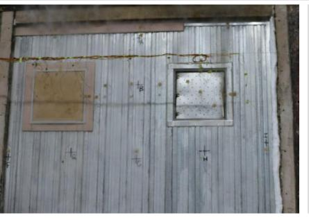
FyreSHIELD™ Plus access panels were independently tested by BRANZ to AS 1530.4:2014, installed in a 78 mm KOROK® wall system. This test was conducted with two panels in a single wall – one installed to face the furnace's fire source directly, and one installed on the opposite side, facing away from the furnace.
