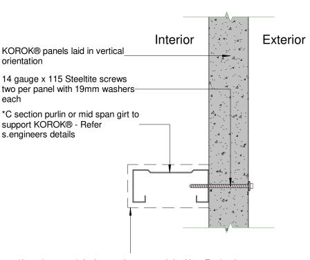
\*In order to satisfy the requirements of the New Zealand Building Code (clause C6) relating to "structural stability during fire" designers must ensure that KOROK® elements are supported by primary elements that have at least the same fire rating as the KOROK® system that is used.
