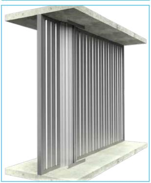
12 Panels must be screwed together into every panel joint as per the vertical centres in Table 3 below.
