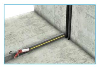
Using a masonry drill bit, pre-drill the C-track at 400mm centres.
