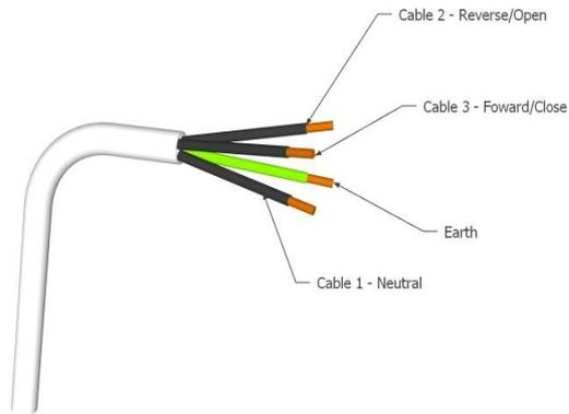
1. Black wires have numbers printed on the plastic insulation
