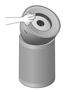
Check the sensor inlets on the left hand side of the conic amplifier for dust and debris.
