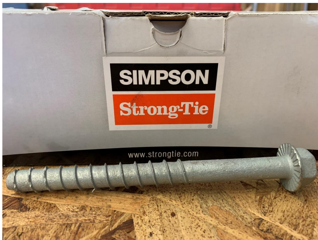
Figure 1. THD 12 x 150 mm screw bolt sample.
