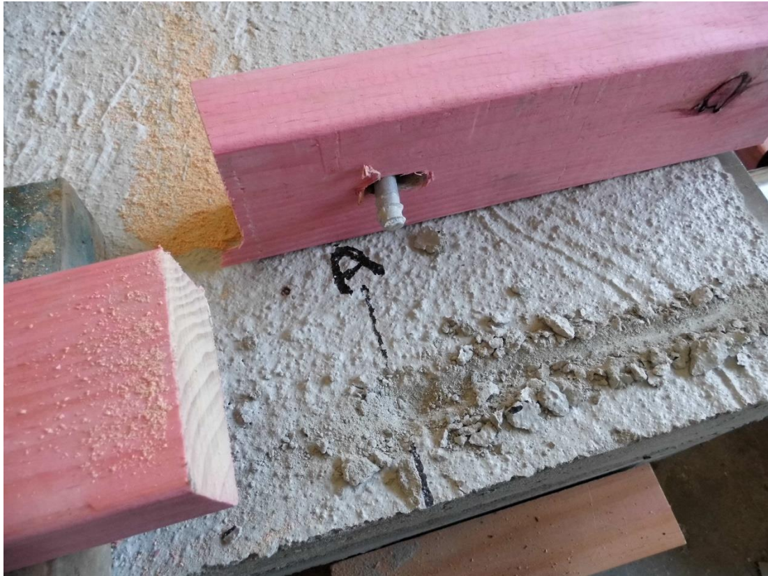
Figure 8. In-plane shear, typical anchor shear failure.
