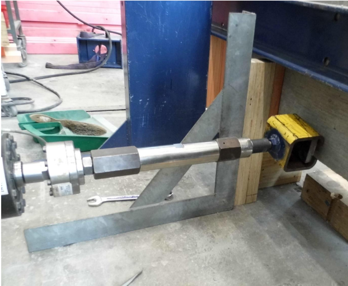
Figure 6. Load applicator for the tensile tests.
