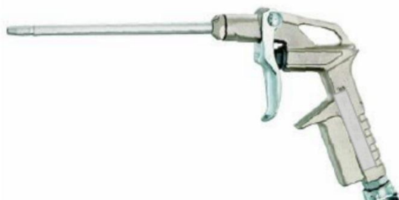
Figure 5: Cleaning air gun. Suitable min pressure 6 bar at 6 m 3 /h. Oil-free compressed air. Recommended air gun with an orifice opening of minimum 3.5 mm diameter
